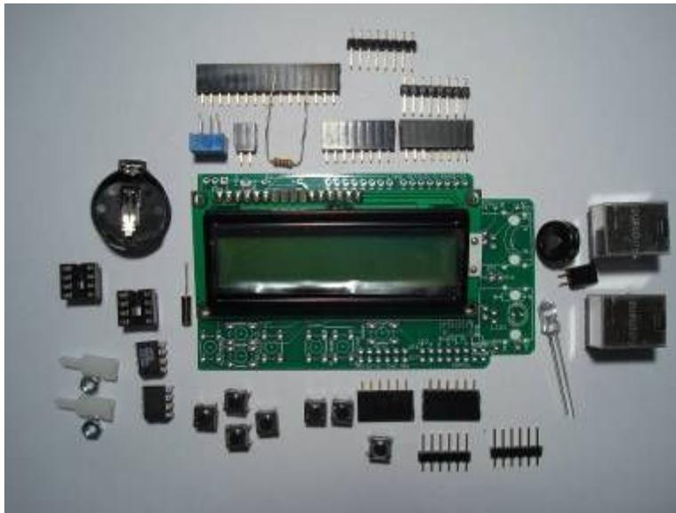
Fig. 1 Unassembled shield with all parts.
