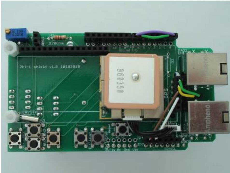
Fig. 9 A shield with an EM 406A GPS module (LCD is removed to show the GPS)
